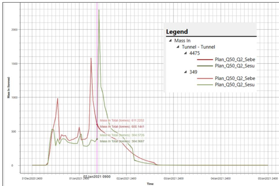
**Figure 16.** Comparison of the amount of sediment transport (tons) entering the inlet and tunnel outlets in the design flood conditions of Q50, before and after normalization
