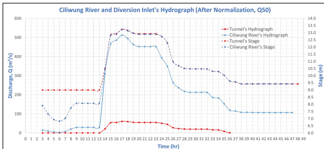
**Figure 7.** Hydrograph of Ciliwung River and Diversion Tunnel
