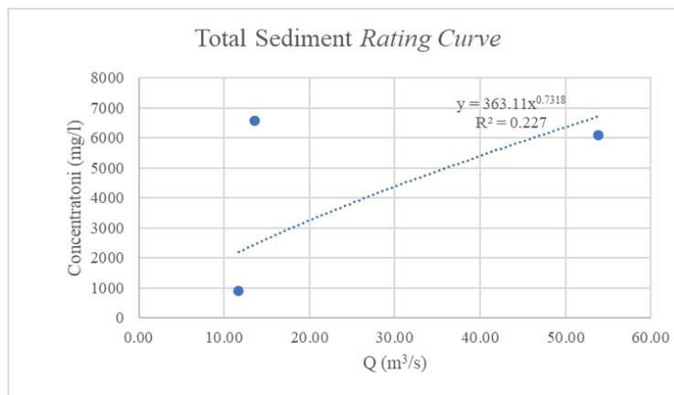
Figure 10. Total Sediment Rating Curve
