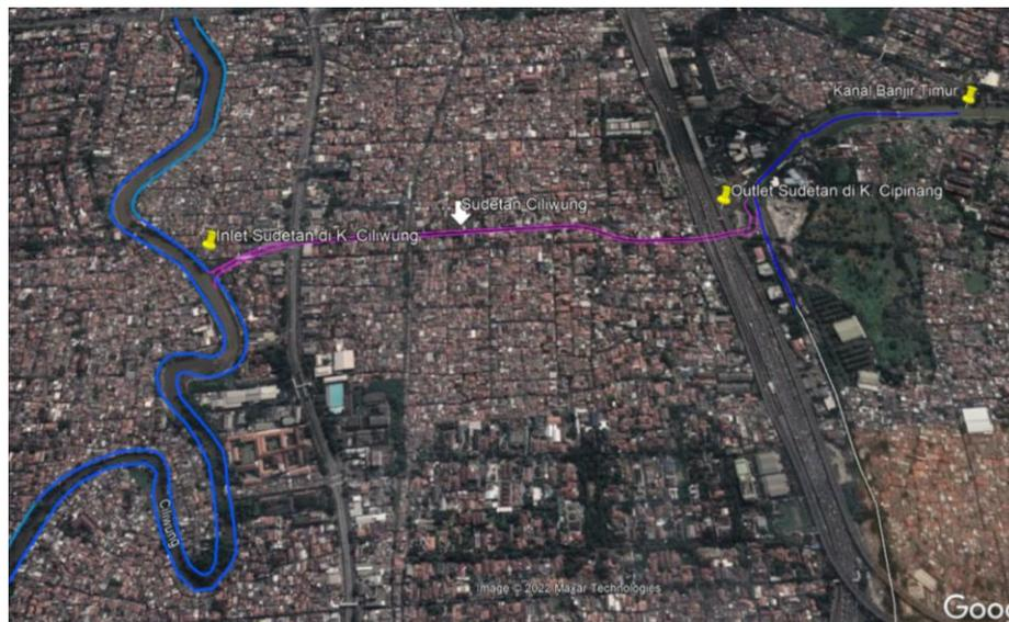
**Figure 1.** Layout of Ciliwung - KBT diversion system
