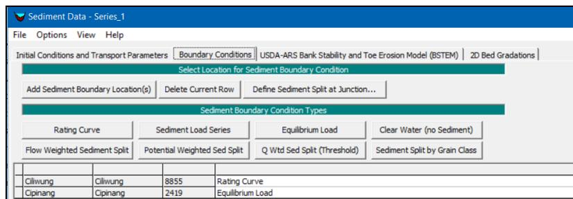
**Figure 14.** Sediment boundary conditions for diversion system model
