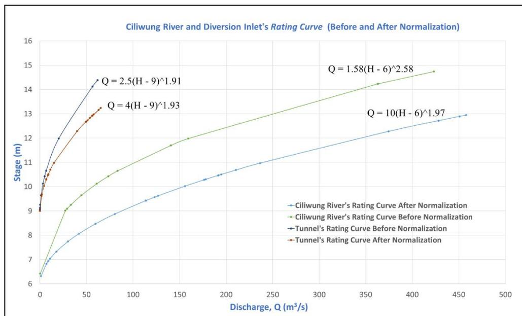
Figure 6. Rating Curve of Ciliwung River and Diversion Tunnel
