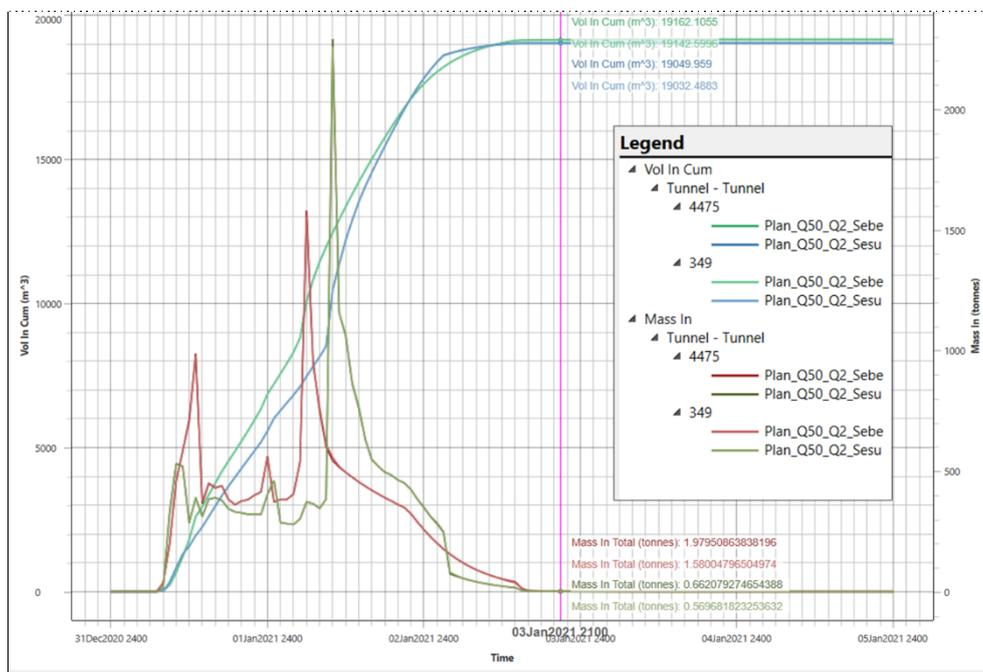
**Figure 17.** Graph of the comparison of the mass of incoming sediment with its cumulative volume at the inlet and outlet of the drain, before and after normalization
