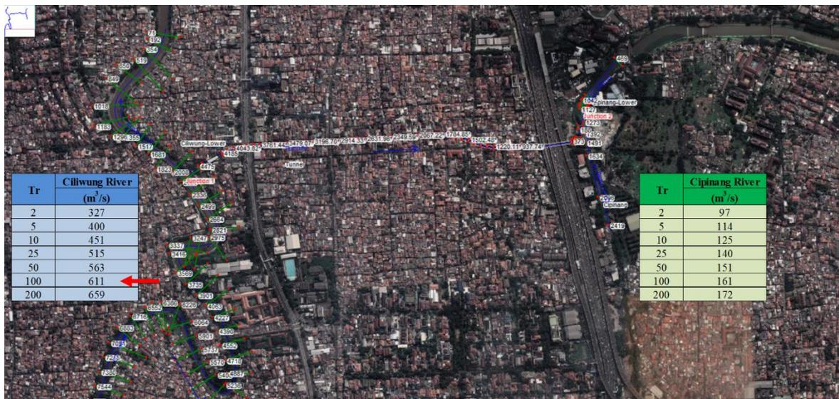
**Figure 12.** Schematic of the Ciliwung River – Diversion Tunnel – Cipinang River – KBT, with a Google Map background
