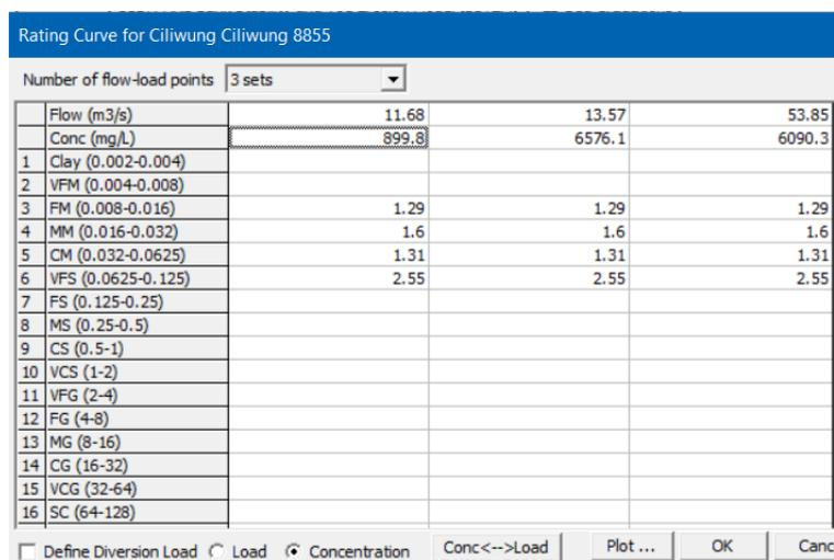
**Figure 15.** Rating Curve used as sediment boundary condition
