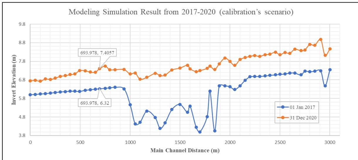
**Figure 11.** The Ciliwung’s invert elevation at the inlet location, modeling simulation result from the 2017-2020
