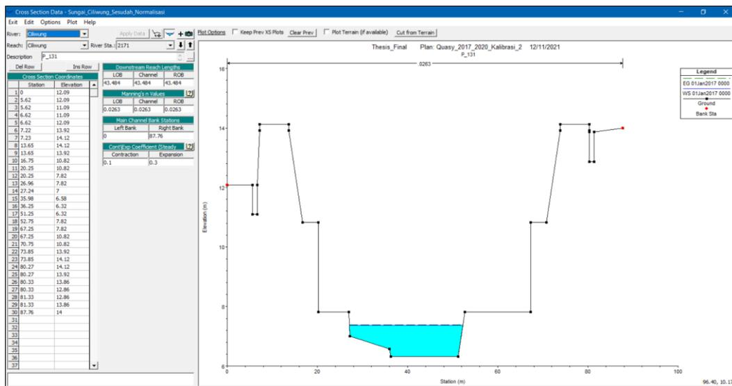
Figure 9. Geometry display of Ciliwung River model calibration scenario
