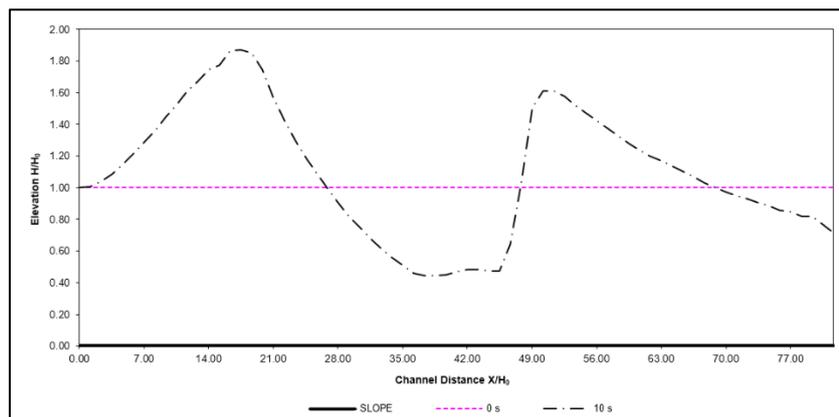
**Figure 10.** Distribution of water depth along the wall for 10 seconds simulation
