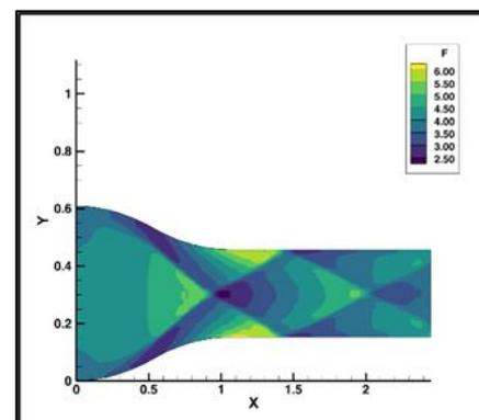
**Figure 7.** Contour of Froude number for 10 seconds simulation
