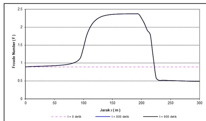
**Figure 6.** Longitudinal profile of 2-terrace hydraulic jump case of Froude number
