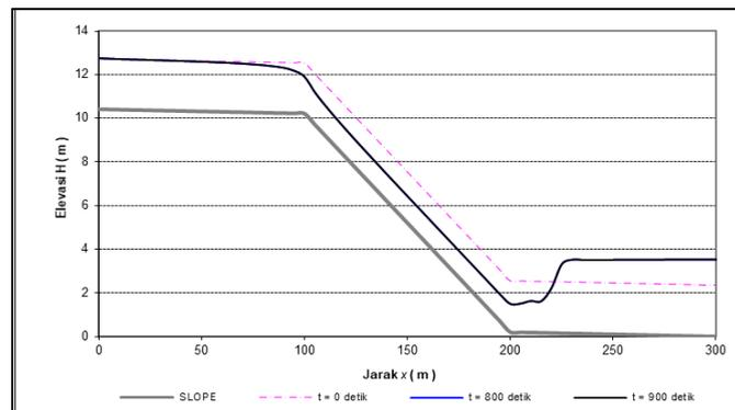
**Figure 5.** Longitudinal profile of 2-terrace hydraulic jump case
