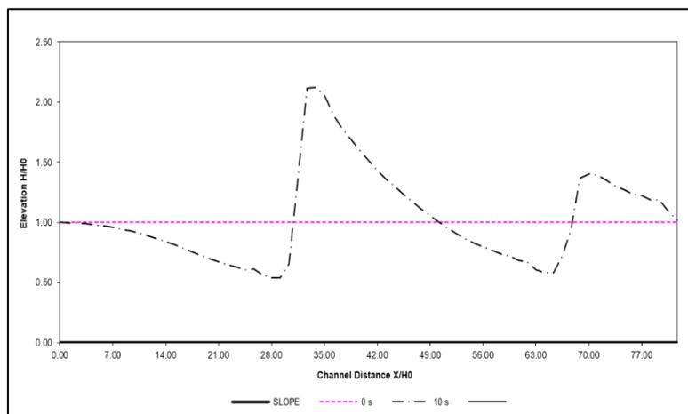
**Figure 9.** Distribution of water depth along center for 10 seconds simulation
