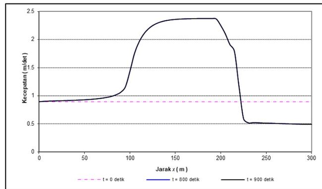
**Figure 7.** Longitudinal profile of 2-terrace hydraulic jump case of velocity flow
