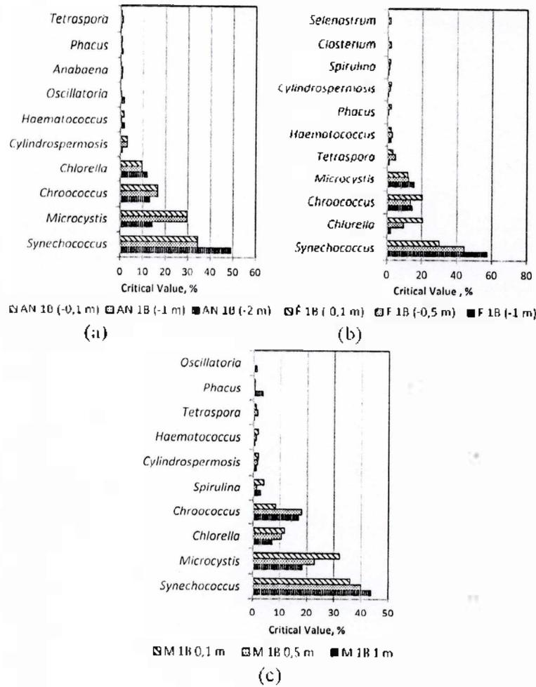
Figure 7. Profiles of critical values microalgae genera diversity in (a) anaerobic, (b) facultative, and (c) maturation pond of stabilization ponds set 1B Bojongsoang WWTP
