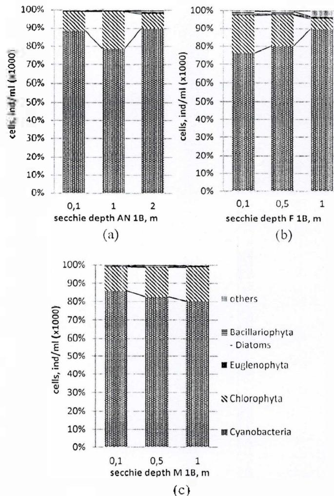
Figure 6. Profiles of microalgae diversity in (a) anaerobic, (b) facultative, and (c) maturation pond of stabilization ponds set 1B Bojongsoang WWTP
