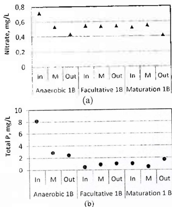
Figure 3. Profiles of (a) nitrate and (b) total phosphate concentrations of stabilization ponds set 1B Bojongsoang WWTP
