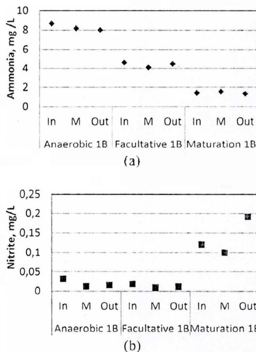
Figure 2. Profile of (a) ammonia and (b) nitrite concentrations of stabilization ponds set 1B Bojongsoang WWTP
